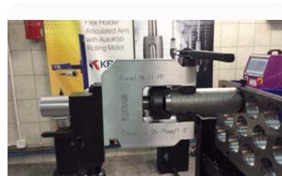
Inconel cladding removal application on 1" length
