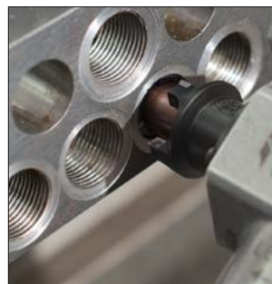
Safely re-machine gasket surfaces in seconds.
